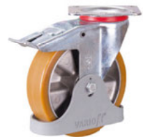
Polyurethanrolle 92° Shore A Traglast 2000 kg
